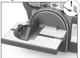
Figure 10. Squaring the miter gauge.
